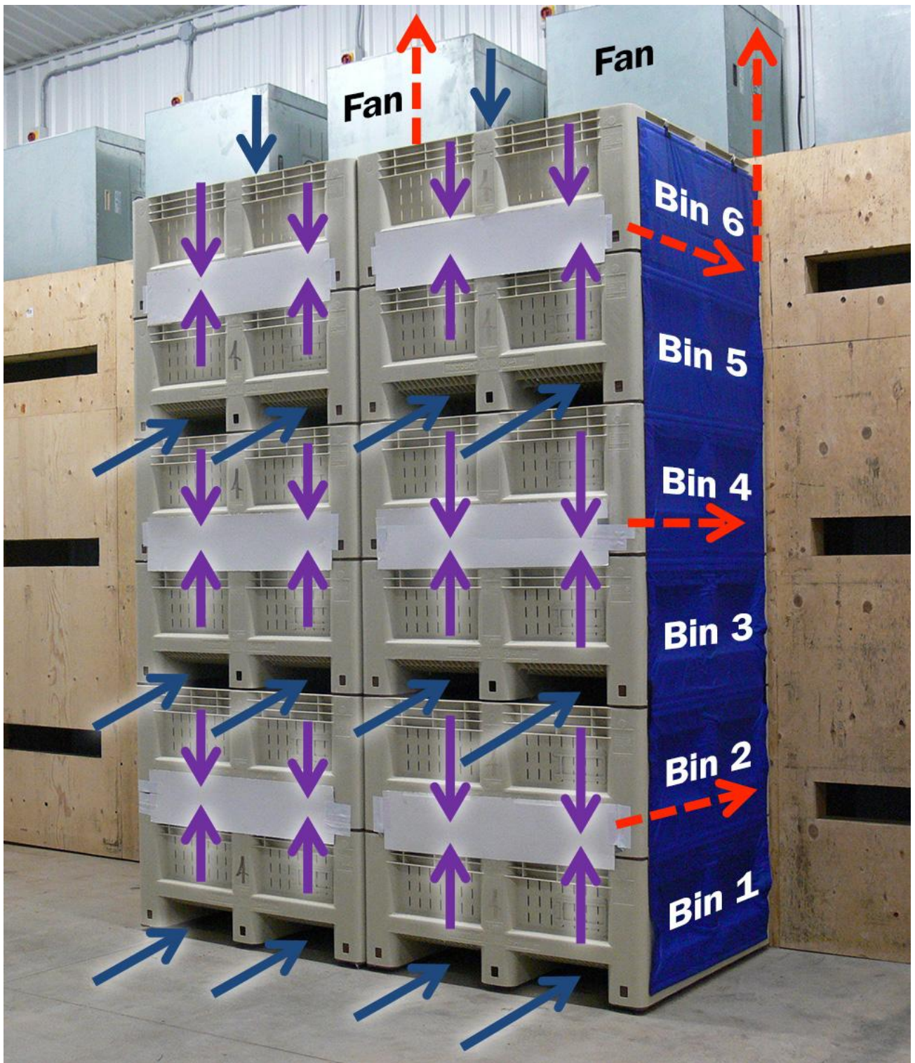
Figure 4. This serpentine horizontal/vertical airflow system has centrifugal fans inside metal housings above a plywood plenum. These fans pull refrigerated air through “hot” tree fruit in plastic bins. Each stack of six bins is independent. Three forklift openings across from wall slots are closed off with coverings. This compels cold air to enter through the remaining three open forklift openings and travel up or down through the fruit via slots in the bin floor. As the air
